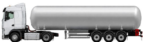
28–37T road tanker
